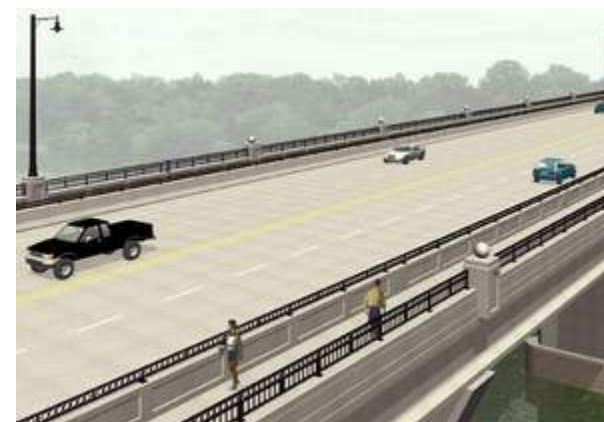
The new College Avenue bridge will be 1,372 feet long and 54 feet wide. It will be made of 1.3 million pounds of reinforcing steel. Submitted illustration
